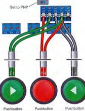
Normally Closed Normally Open Normally Open "Stop" "Run Reverse" "Run Forward" [Order Codes 29992 x 2, 29989, 30409 x 3, 30477, 30146 x 2]
